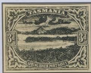
3d Spring River Zinc block after etching, before asphaltum removal. Note black clouds.
