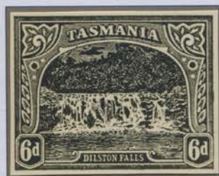
6d Dilston Falls Zinc block after etching, before asphaltum removal. Note dark trees.
