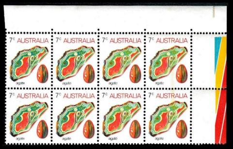
If the doctor blade is set too firmly it can wipe the ink from the etched cells leaving a paler than usual colour. The right two columns show a paler green due to the scooping out of the yellow.
