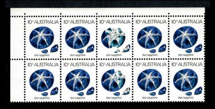
On rare occasions some foreign matter will get between the paper sheet and the ink cylinder. When the foreign matter is removed a void is left on the printed stamps.
