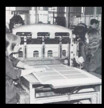
The printed sheets are then checked for printing errors using the colour bars at the edge of each sheet. They are then perforated and guillotined into smaller sheets for issue to the post office.
