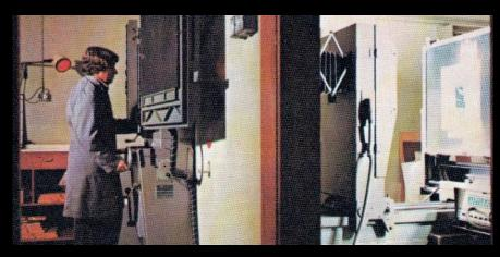
Finished artwork for each colour is transformed into a large multipositive – the same size as a printed sheet of stamps.
