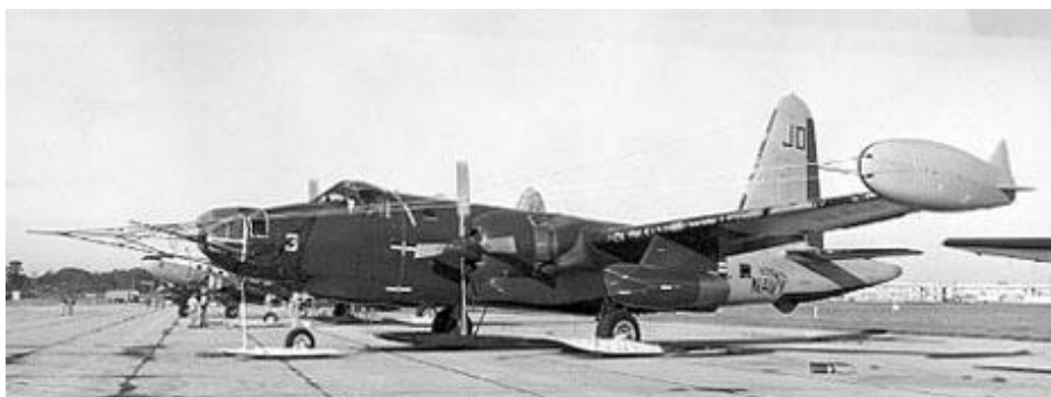
LP-2J, 140439 fitted with the Fulton Skyhook Retriever System
